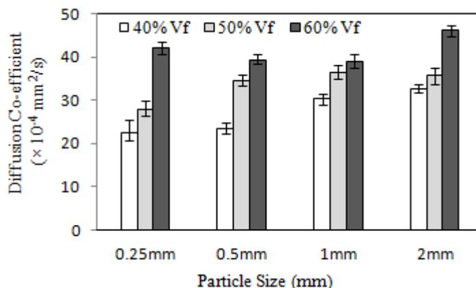
Figure 2: Diffusion Co-efficient of CSPE composite samples
