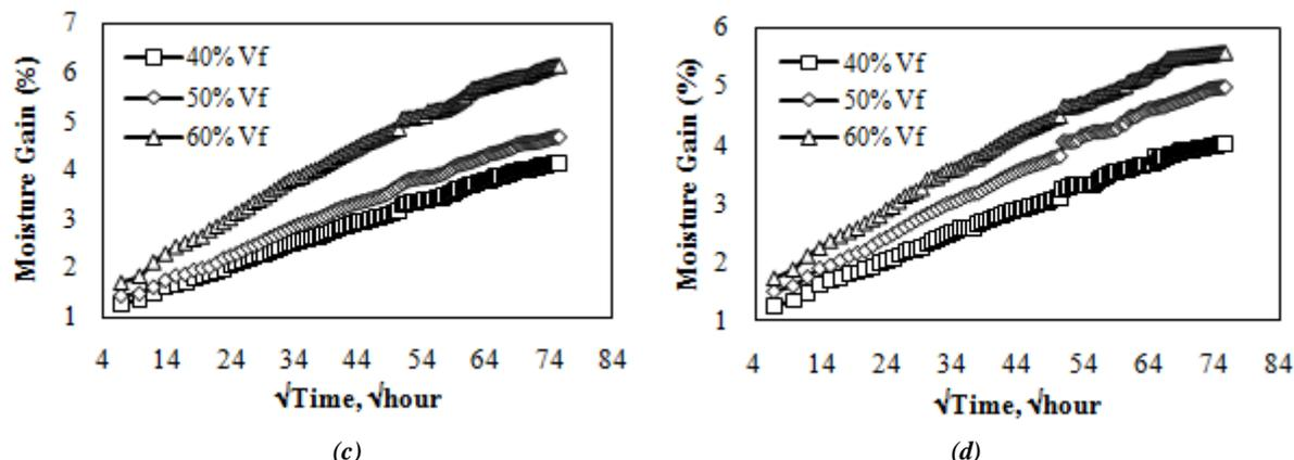
Figure 1: % Moisture Gain V/s root of time curve for CSPE Composites with (a) 0.25mm PS (b) 0.5mm PS (c) 1mm PS (d) 2 mm PS in different filler volume fraction (Vf).
